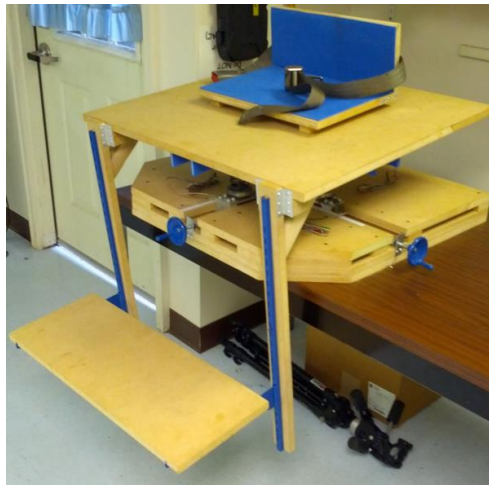
Figure 5.3: The prototype design uses strain gauges instead of a force plate to track the user's movements.
